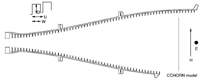
FIG. 2. Profile of the 10 GHz horn as designed, with a close-up showing dimensional parameters. The extent of the modeled unsliced horn is shown, as are the directions of the *E* and *H* planes as referred to in the article.
