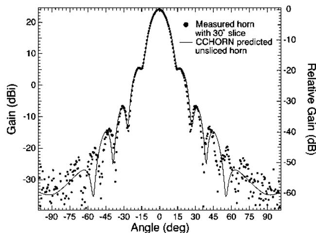
FIG. 4. Predicted and measured  $E$ -plane beam pattern for the 10 GHz horn at 10.11 GHz.
