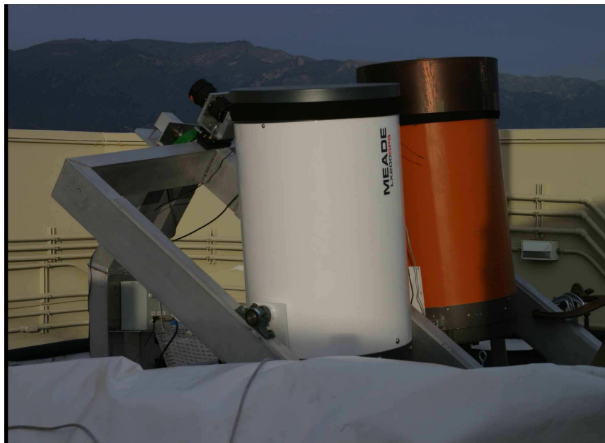
Fig. 1. Celestron (14 inch aperture, f/11) and MEADE (16 inch aperture, f/11), on aluminum mount.
