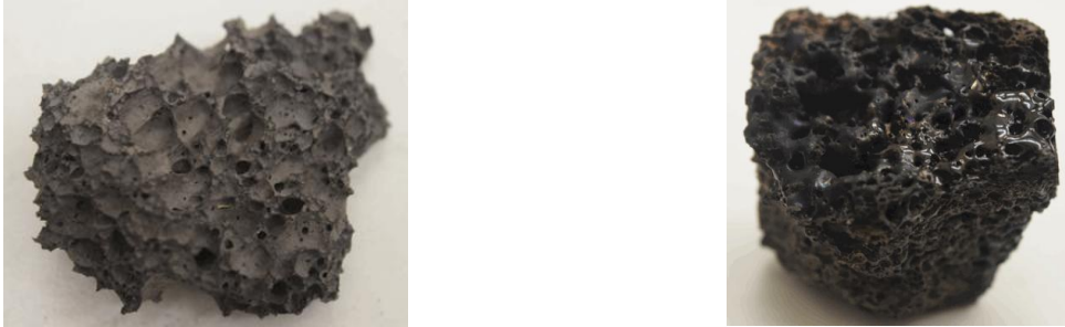
Figure 8. Porous basalt sample that has not undergone any ablation ( Left ). Sample of basalt from lab testing that has undergone ablation ( Right ). Both samples come from the same basalt rock.
