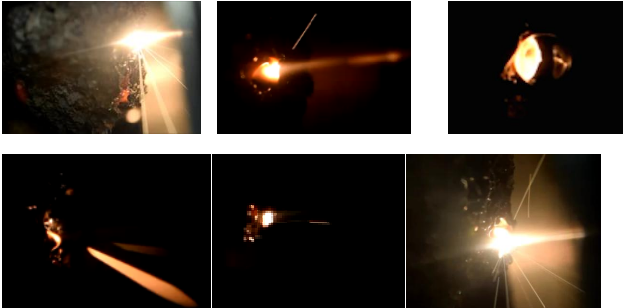
Figure 16. Various pictures of mass ejecta, sparks, plume, and bubbles due to laser ablation. These pictures show the environment at the sample while laser ablation is occurring. See online video.
