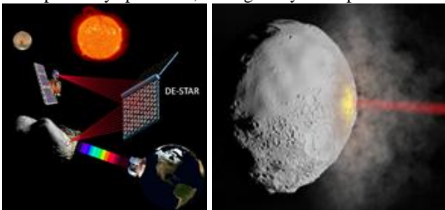
Figure 1. Left: Concept diagram of an orbiting DE-STAR engaged in multiple tasks including asteroid diversion, composition analysis and long range spacecraft power and propulsion. Right: Visualization with relevant physical phenomenon included at a flux of about 10 \text{ MW}/\text{m}^2 . Plume density is exaggerated to show ejecta. Asteroid diameter is about that of Apophis (325 m) relative to the laser beam diameter (30 m). Target is at 1 AU.
