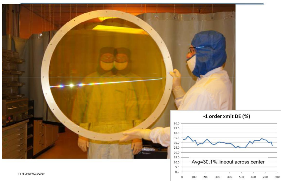
Figure 12 – Thin film replicated optics from DARPA MOIRE Ball-LLNL program. The thin ( \sim 30 micron) plastic film is replicated from an etched mandrel. Areal mass of the film is approximately 60 \text{ g/m}^2 with actual optical mass dominated by mounting ring and not the optic itself. Thin glass and other materials are other possibilities for these lightweight replicated optics. In our system all optical elements are identical leading to mass production replicated techniques being optimal.
