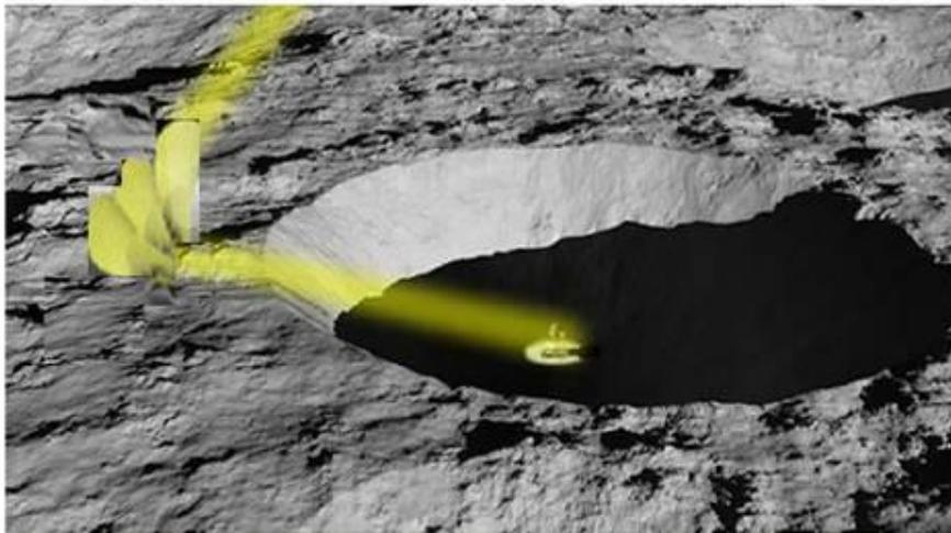
The ER starts its descent into the crater. The TF continuously tracks the ER, lighting its path with reflected sunlight. As the ER reaches areas with ambient temperatures below 100K, it is powered and warmed by the TF projected energy.
