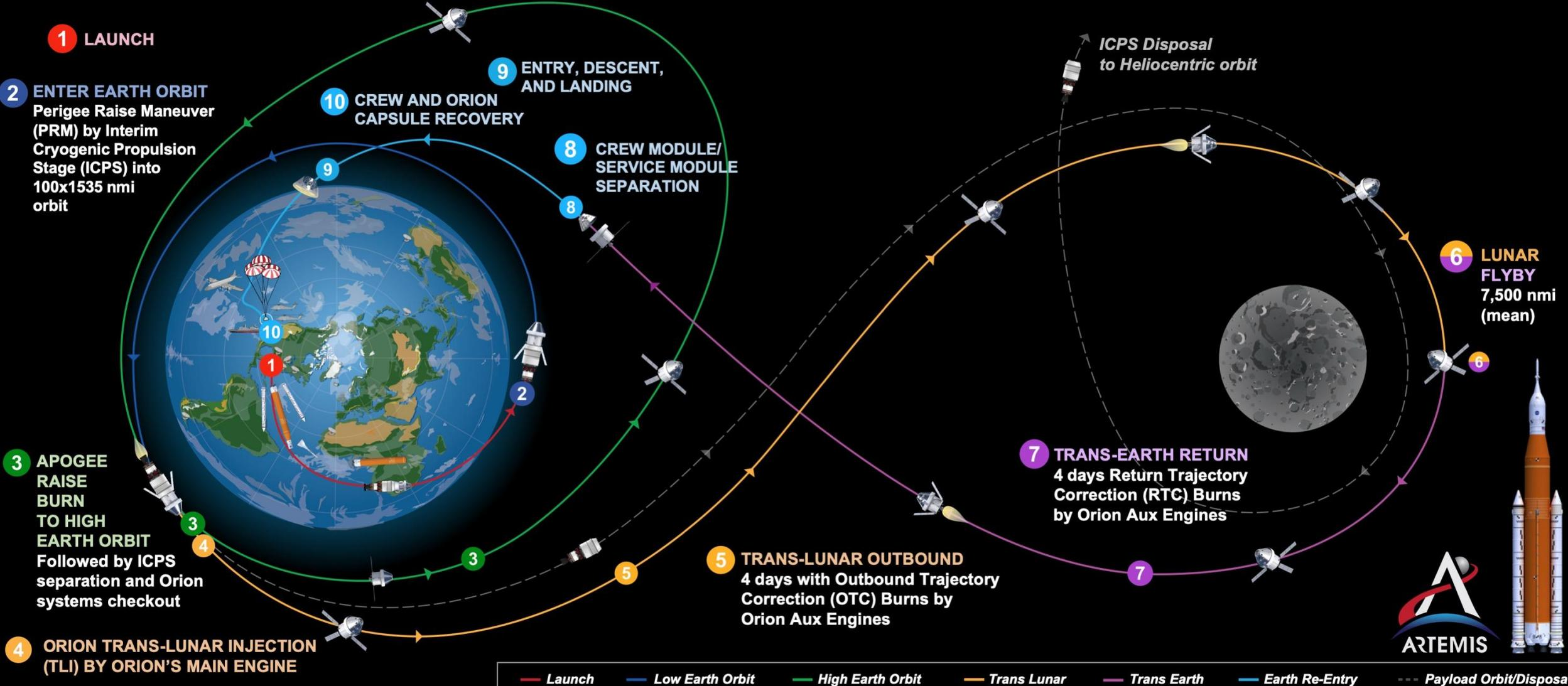
SLS Configuration (Block 1) with Human Rated ICPS | 15x1200 nmi insertion orbit | 28.5 deg inclination
