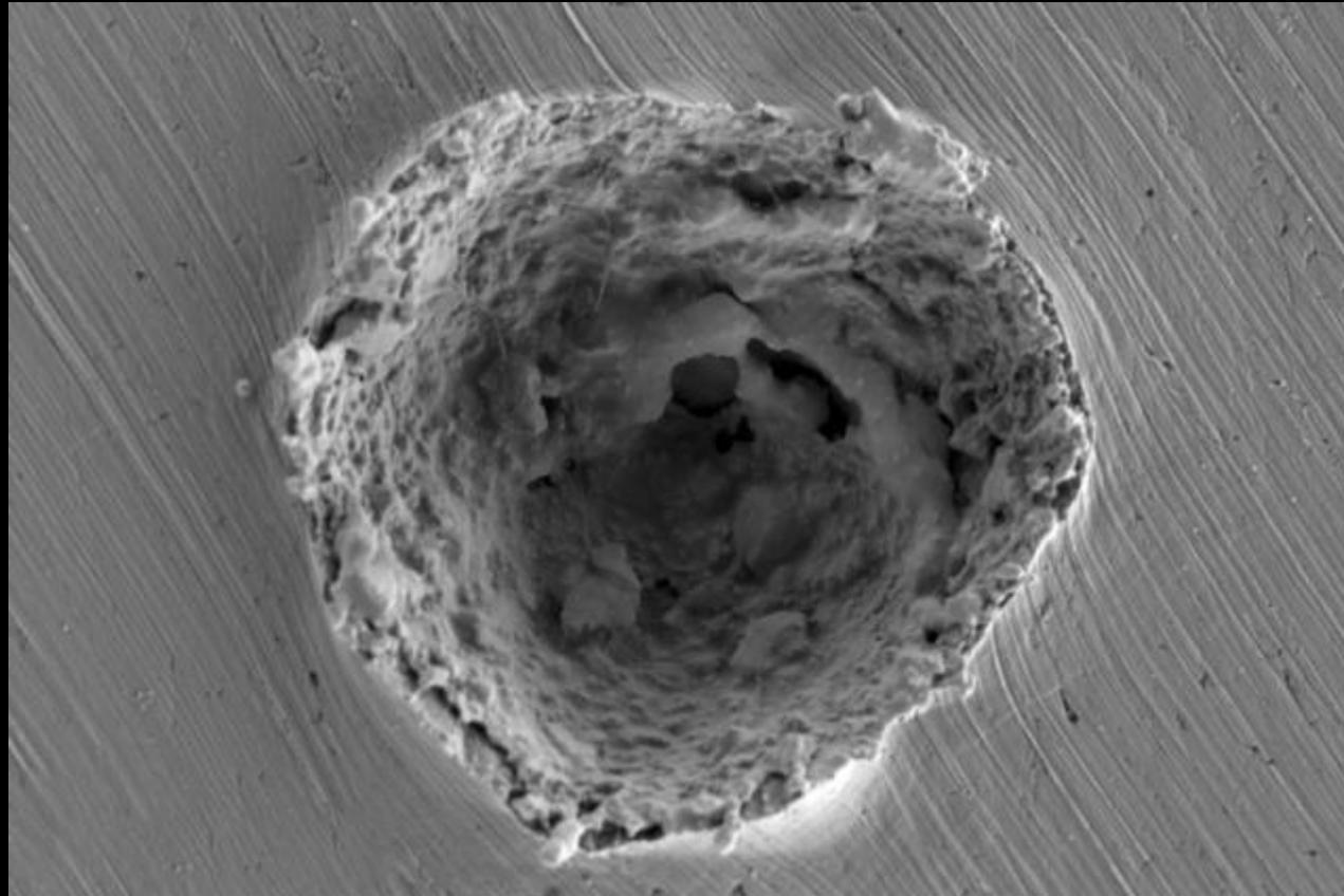
**Micrometeorite damage to a surface in LEO. Similar damage can occur on the Moon where micrometeorites land at upwards of 10 km/second.**
