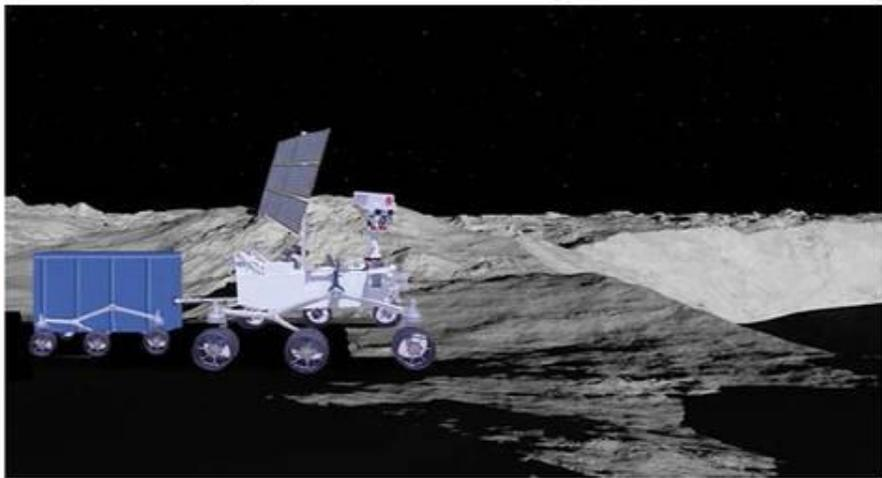
The rover makes its way out of the landing module, transporting a compactly folded TF, and approaches the rim.
