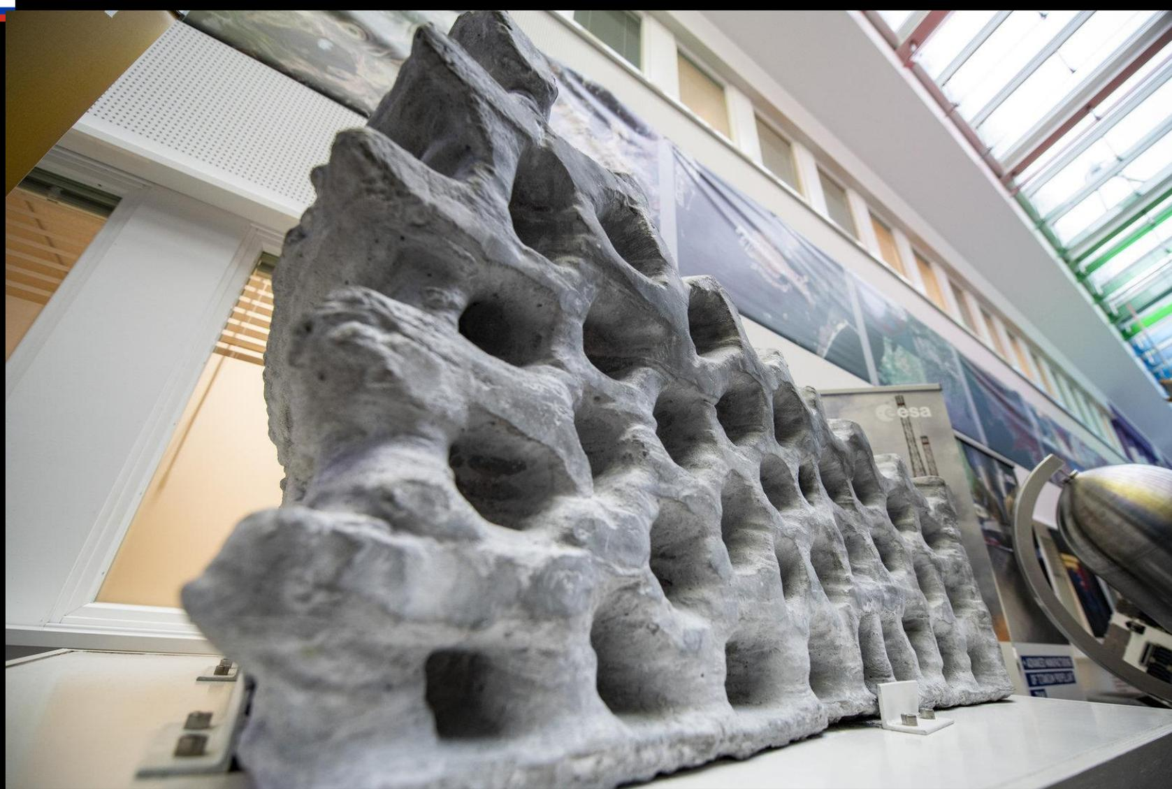
**1.5 metric ton block at ESTEC in Noordwyk was 3D printed from lunar regolith simulant.**
