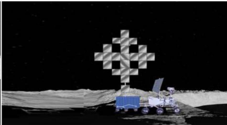
The TF unfolds to reflect sunlight into the crater—it is placed at a location that provides line-of-sight coverage of the planned ER path, and, under its own actuation, adjusts its position/posture for improved stability. A crosslet origami unfolding is depicted.
