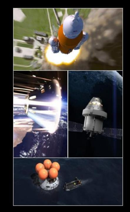
The SLS core stage, the largest rocket stage ever built by NASA, 212 feet tall, 27.6 feet in diameter. Propellant tanks hold a total of 733,000 gallons of liquid oxygen and liquid hydrogen to fuel the four RS-25 engines during launch.
