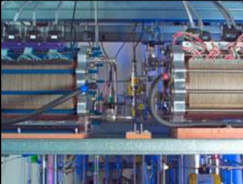
Regenerative fuel cell stacks at NASA Glenn. Credit: NASA
