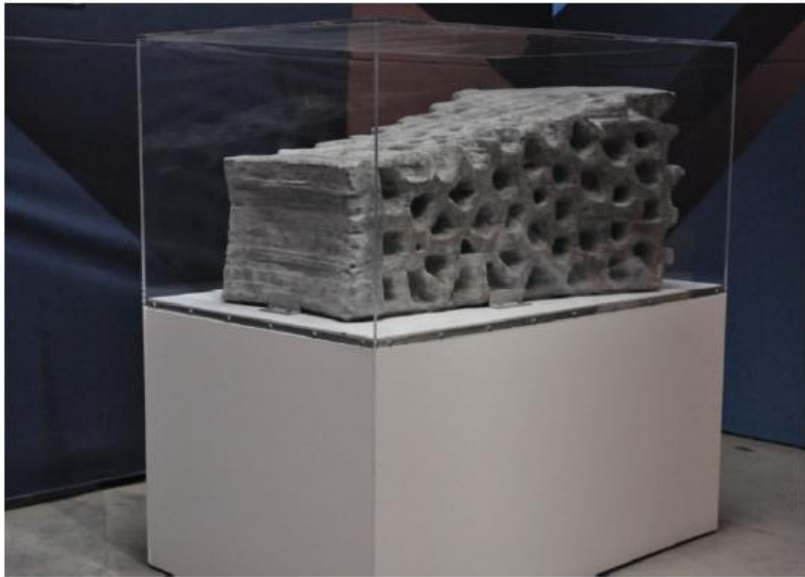
Fig. 26. The 3D-printed structure made of simulated regolith on display at the exhibition entitled "Stazione Futuro", Turin, March-November 2011. Photo: authors
