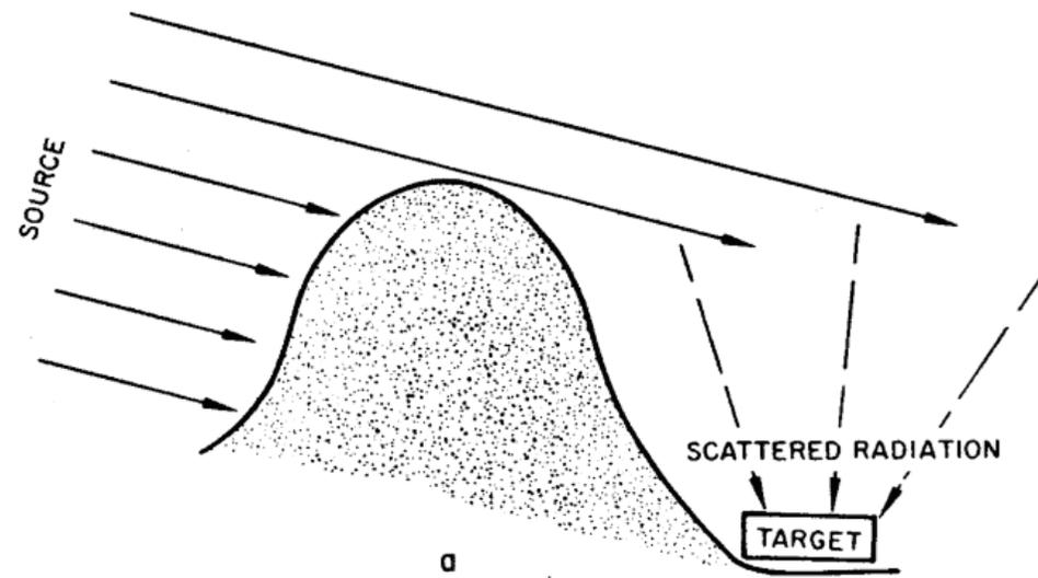
Figure 8.45a. Target exposed to scattered gamma radiation.
