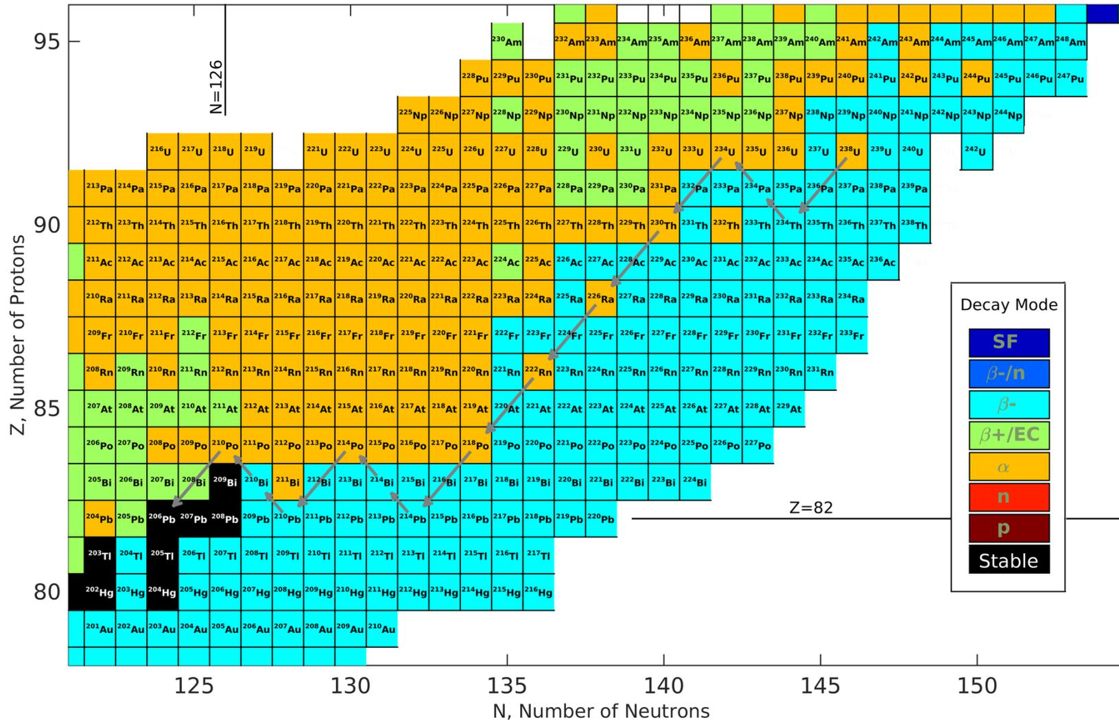
**Example: The uranium-238 series (grey line)** is a series of  $\alpha$  (N and Z less 2) and  $\beta^-$  decays (N less 1, Z plus 1) to nuclides that are successively deeper into the valley of stability. The series terminates at lead-206, a stable nuclide at the bottom of the valley of stability.
