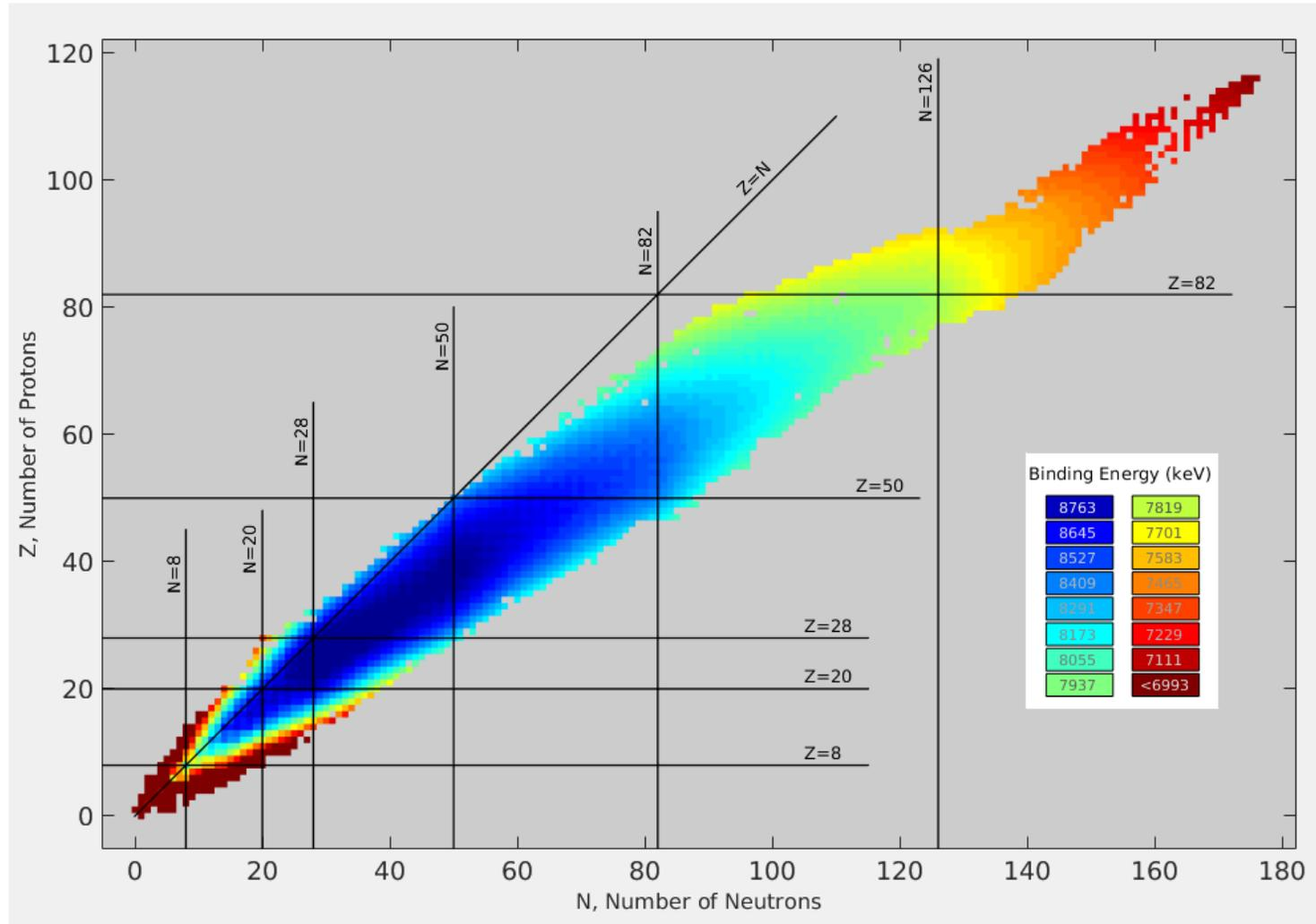
**Chart of nuclides (isotopes) by binding energy, depicting the valley of stability.** The diagonal line corresponds to equal numbers of neutrons and protons. Dark blue squares represent nuclides with the greatest binding energy, hence they correspond to the most stable nuclides. **The binding energy is greatest along the floor of the valley of stability.**
