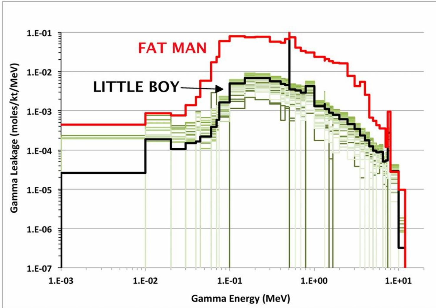
**Figure 3: Gamma spectra for Fat Man and Little Boy. The total Little Boy output (sum over all angles) is shown along with the 40 individual segment tallies scaled up to the full sphere. The segment tallies illustrate the two-dimensional variation of the output.**
