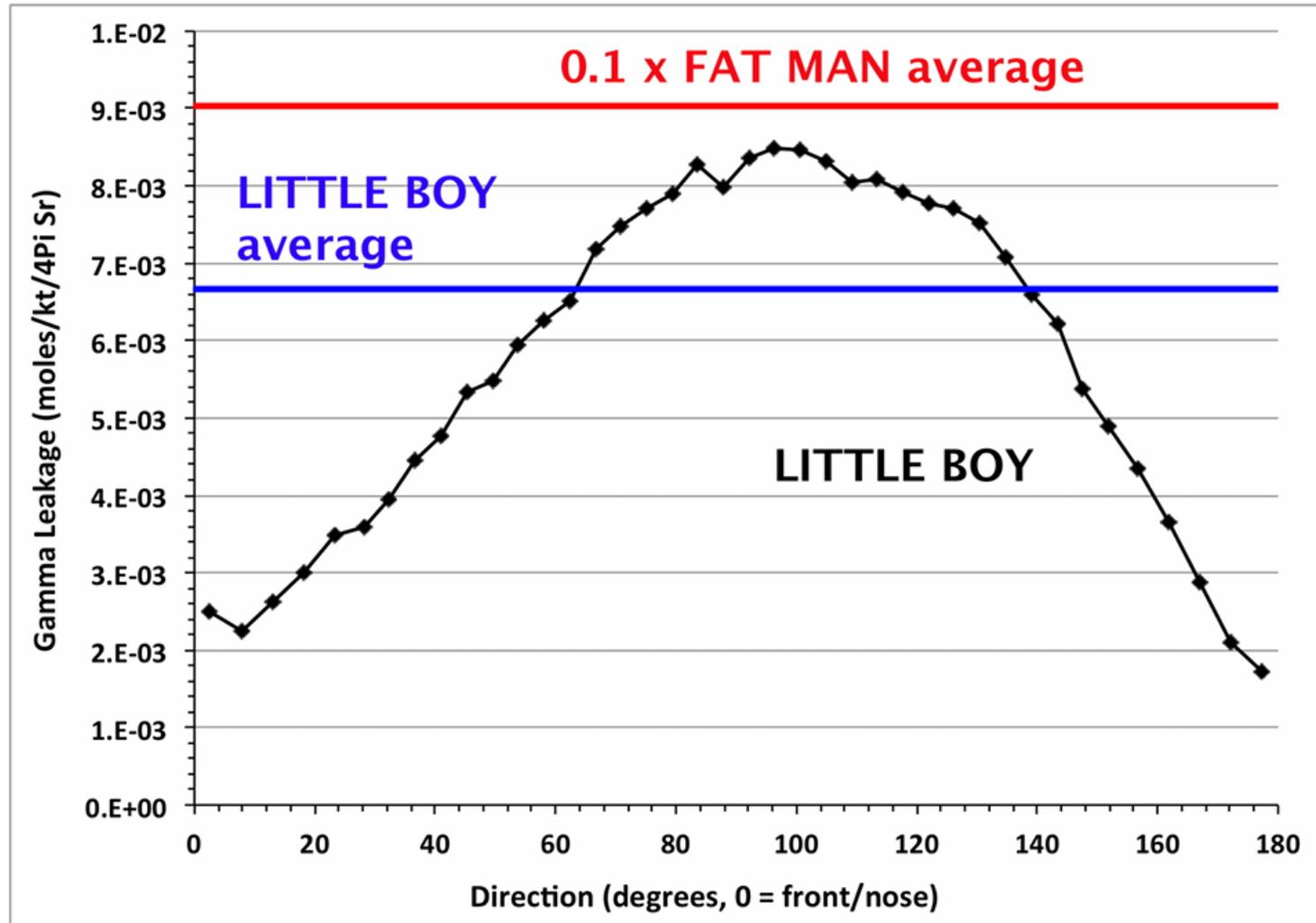
**Figure 5: Gamma output variation with angle.** Segment tallies have been scaled up to the full sphere. Note that the Fat Man value has been reduced by a factor of 10. As with neutrons, the output is suppressed toward the nose (0°) and tail (180°), though these directions represent a small solid angle and the average is heavily weighted toward the values near the waist (90°).
