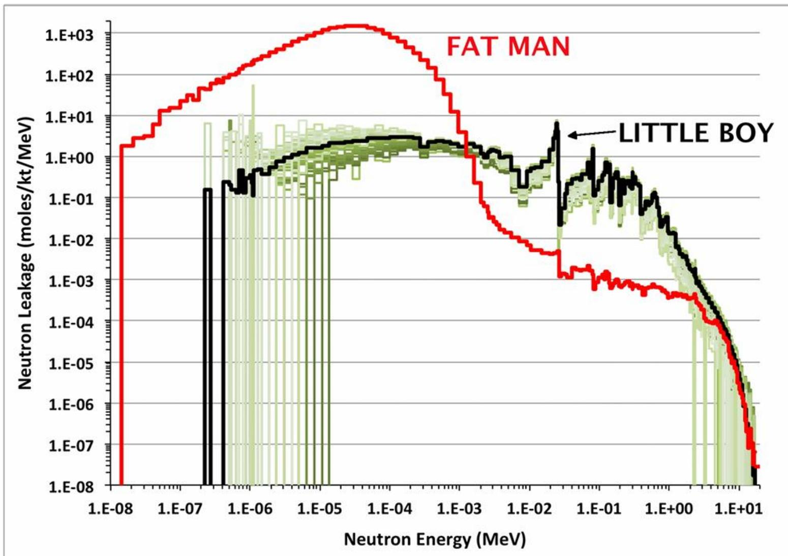
**Figure 2: Neutron spectra for Fat Man and Little Boy. The total Little Boy output (sum over all angles) is shown along with the 40 individual segment tallies scaled up to the full sphere. The segment tallies illustrate the two-dimensional variation of the output.**
