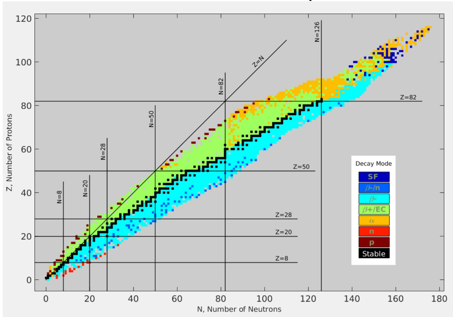
**Chart of nuclides by type of decay mode.** Black squares are stable nuclides. Nuclides with excessive neutrons or protons are unstable to  $\beta^-$  (light blue) or  $\beta^+$  (green) decay, respectively. **At high atomic number, alpha emission (orange) or spontaneous fission (dark blue) become common decay modes.**
