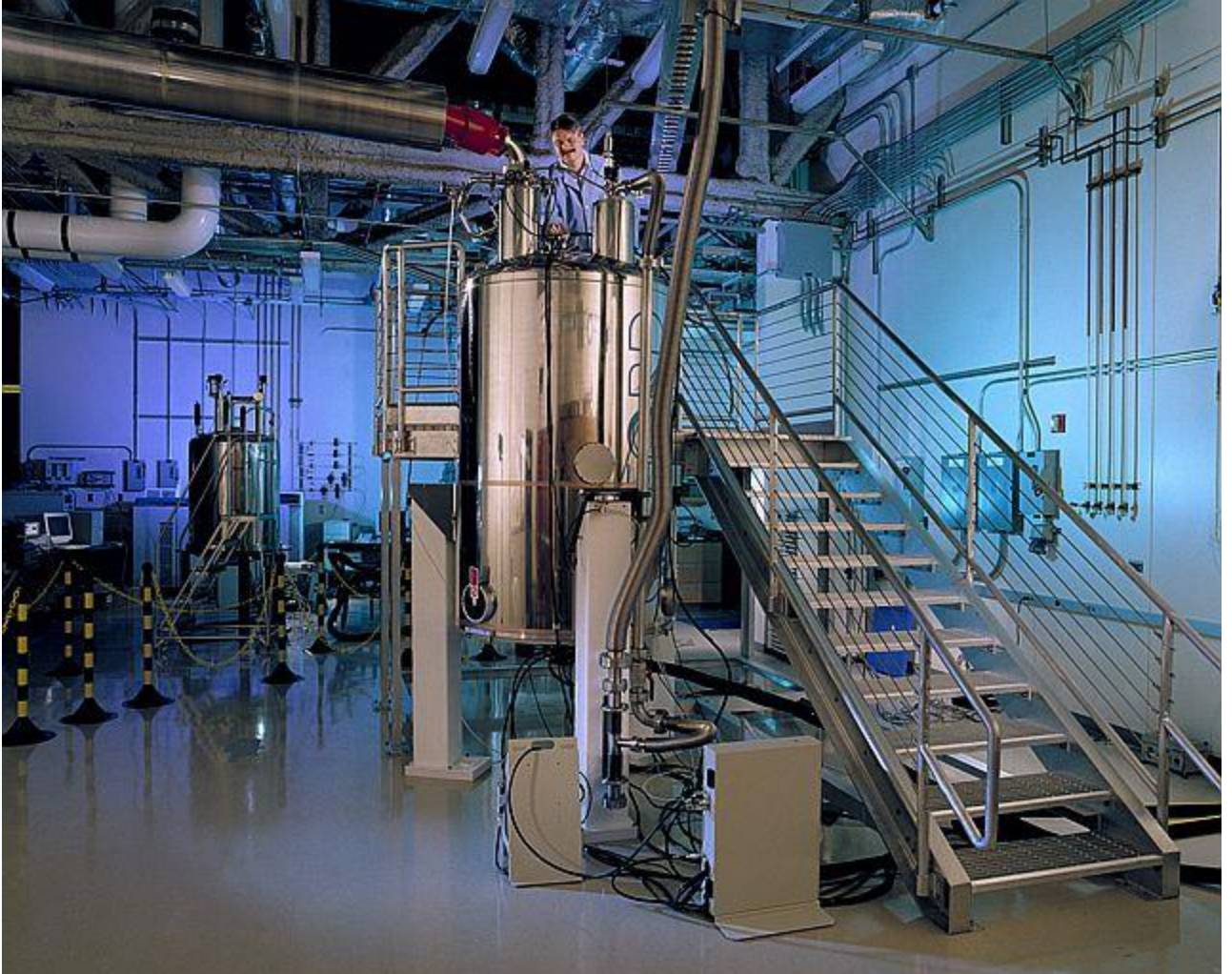
Northwest National Lab – 800 MHz NMR – note superconducting magnet dewar
